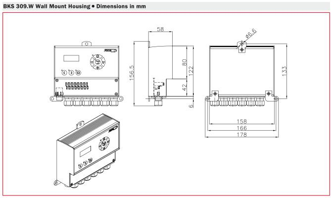
With PG-Gland cable connector. Protection class IP 65.
